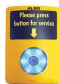
Figure 8: 1202 Call Button – the insert card is interchangeable
