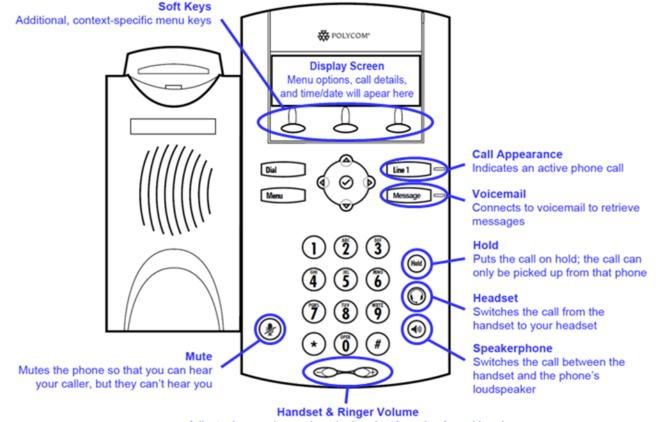
Handset & Ringer Volume Adjusts ringer volume when the handset is on-hook, and handset volume when handset is off-hook
